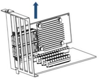
5. When the port connectors reach the top of the chassis window, gently pull the adapter card in parallel to the motherboard.
