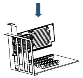
5. When the adapter is properly seated, the port connectors are aligned with the slot opening, and the adapter faceplate is visible against the system chassis.
