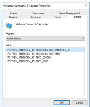
5. In the Value display box, check the fields VEN and DEV (fields are separated by '&'). In the display example above, notice the sub-string "PCI\VEN\_15B3&DEV\_1003": VEN is equal to 0x15B3 - this is the Vendor ID of NVIDIA; and DEV is equal to 1018 (for ConnectX-5) - this is a valid NVIDIA PCI Device ID.
