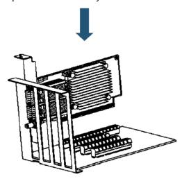
5. When the adapter is properly seated, the port connectors are aligned with the slot opening, and the adapter faceplate is visible against the system chassis.
