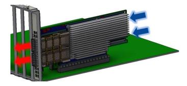
Airflow from the network ports to the heatsink:
